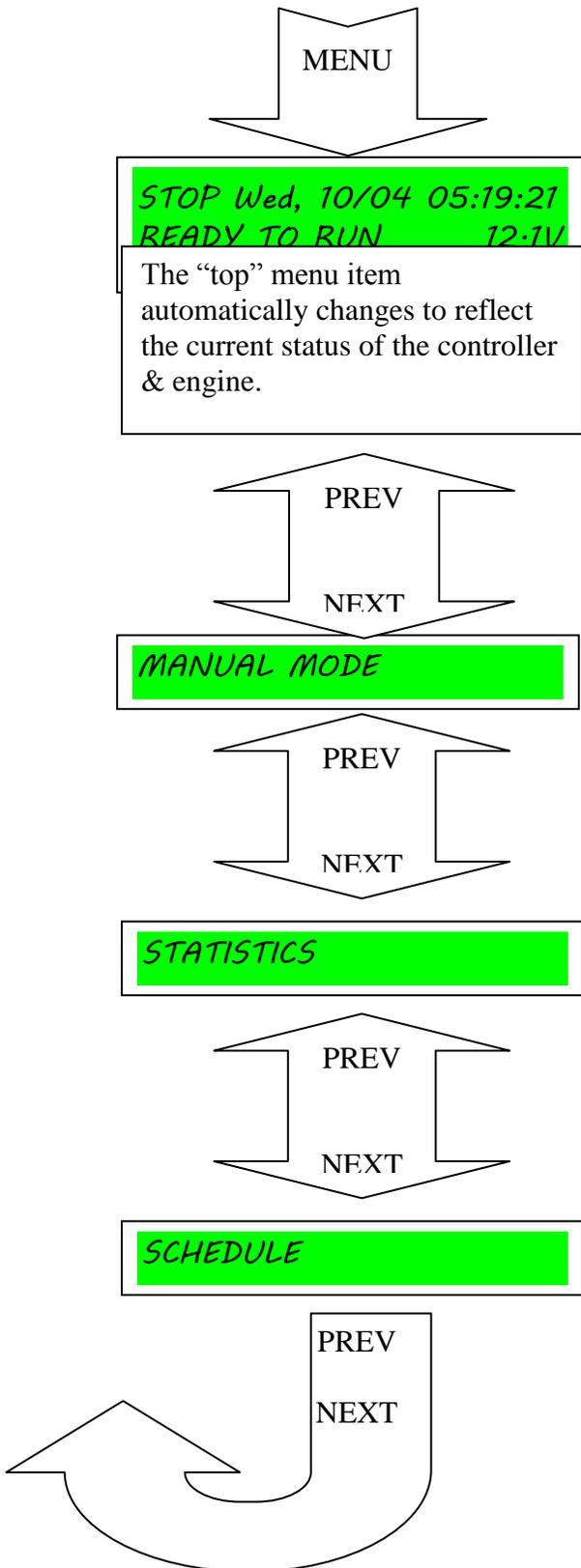
Note: If engine is started without the Controller, then the controller can be "handed" over engine control by going to MANUAL MODE and pressing the SET BUTTON twice – the same as when starting the engine with the controller. The controller will read the engine RPM and recognize that the engine is running. For "powered" ignition engines the ignition switch on the engine should then be turned off so that the controller can shut down the engine.
